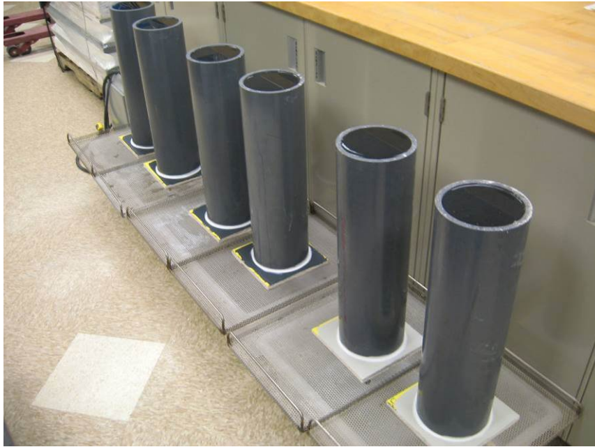
Photo No. 1 Water Resistance Test Set Up
