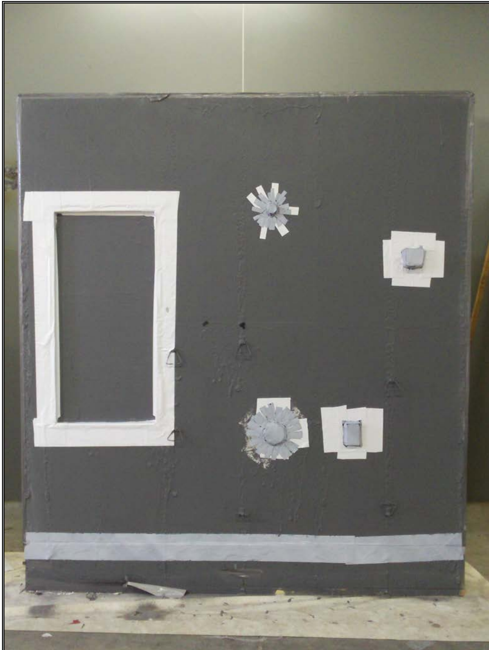
Photo No. 1 Penetrated Wall
