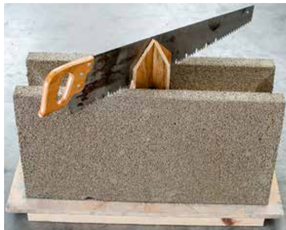
Figure 4: Simple and inexpensive 90° corner jig.
